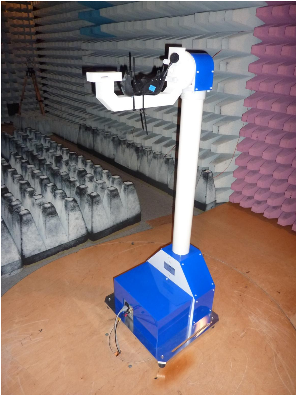
151497_n_f.JPG: FPS COM 7000, test set-up fully anechoic chamber (1 GHz to 5 GHz)
