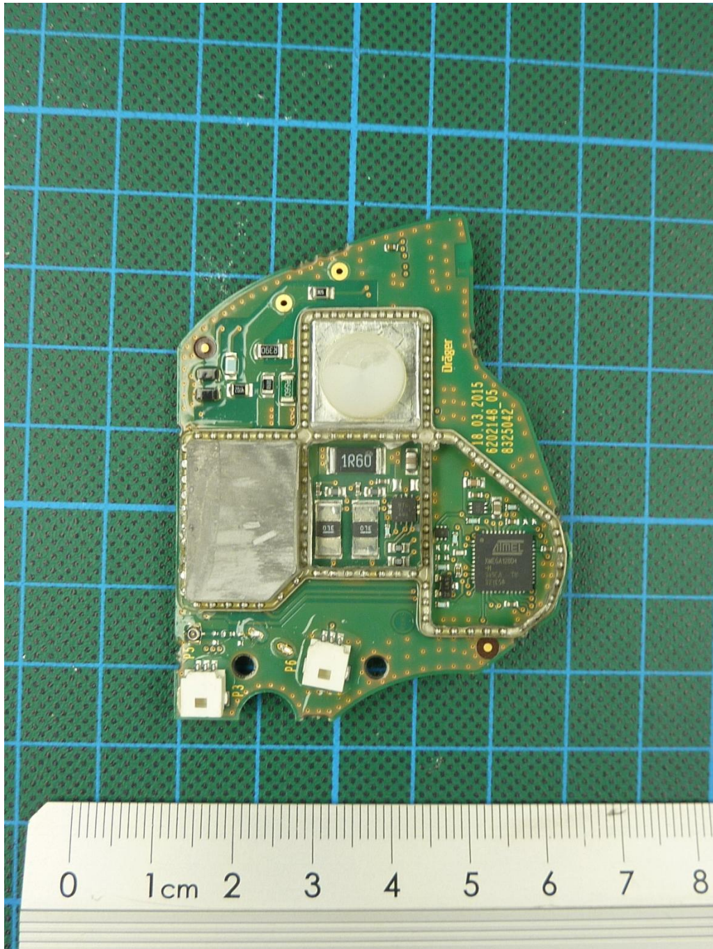
151497_n_9.JPG: FPS COM 7000, PCB2, top view, antenna and shielding removed
