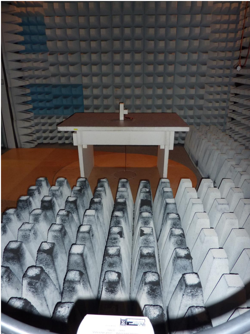
161065_1d.jpg: BT7000, test setup fully anechoic chamber
