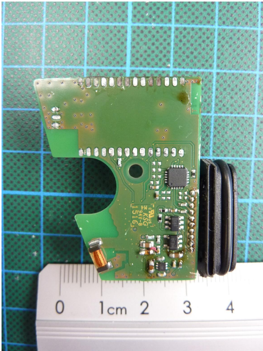
161065_108.jpg: BT7000, PCB, bottom view, Bluetooth module removed
