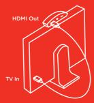
Connect Biscotti "HDMI Out" to the TV using an HDMI cable (not included)
