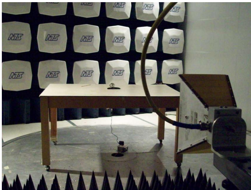
Radiated Emissions 1GHz-6GHz (FCC Chamber), Front of EUT
