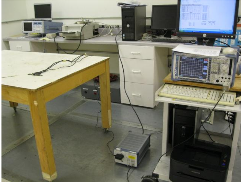
Conducted Emissions Test Setup
