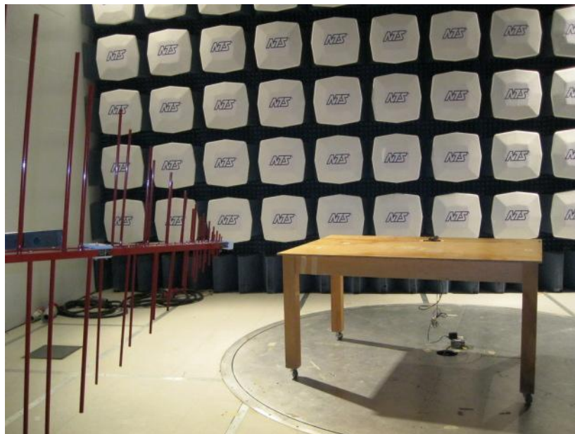
Radiated Emissions 30MHz-1GHz (FCC Chamber), Front of EUT
