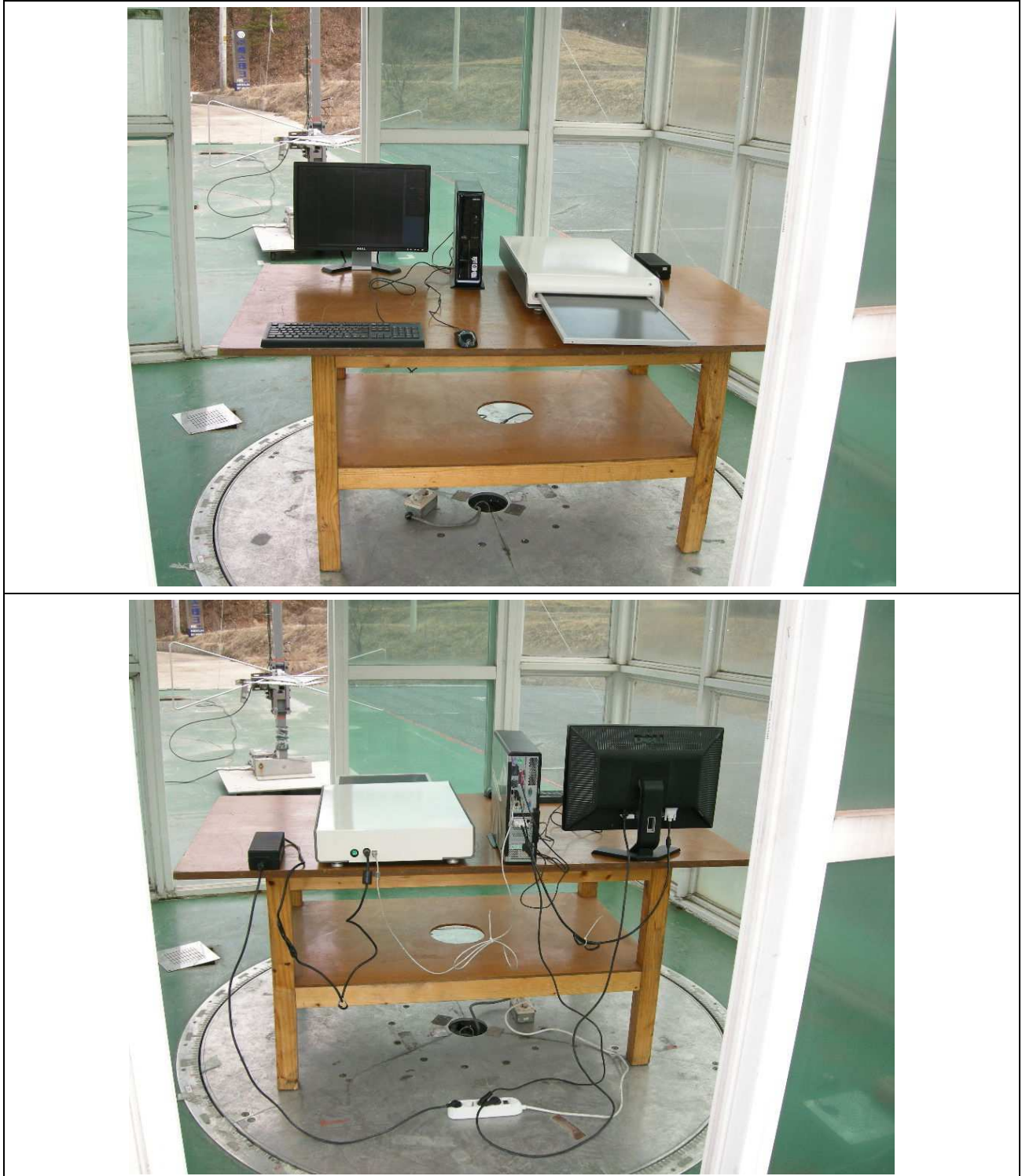
Figure 3. Photo of Radiated emission test setup
