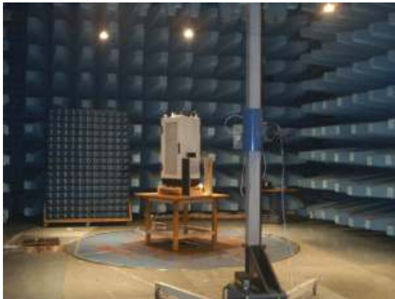
Log periodic antenna 1000 MHz ÷ 5000 MHz) measurement distance: 3 m
