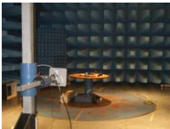
Log periodic antenna 1000 MHz ÷ 10000 MHz) measurement distance: 3 m
