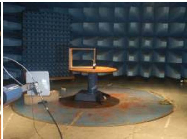
Log periodic antenna 1000 MHz ÷ 10000 MHz measurement distance: 3 m
