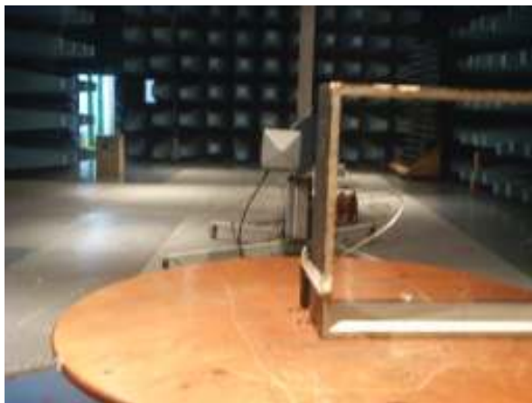
Log periodic antenna 1000 MHz ÷ 10000 MHz measurement distance: 3 m
