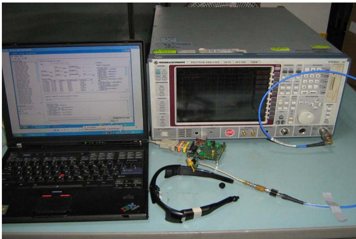
**POWERLINE CONDUCTED EMISSIONS MEASUREMENT SETUP**
