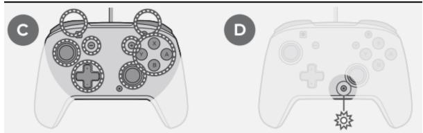
Press the button who's function you would like to assign to the back button. The "function" button's LED will flash 3 times, indicating a successfully mapped function.
