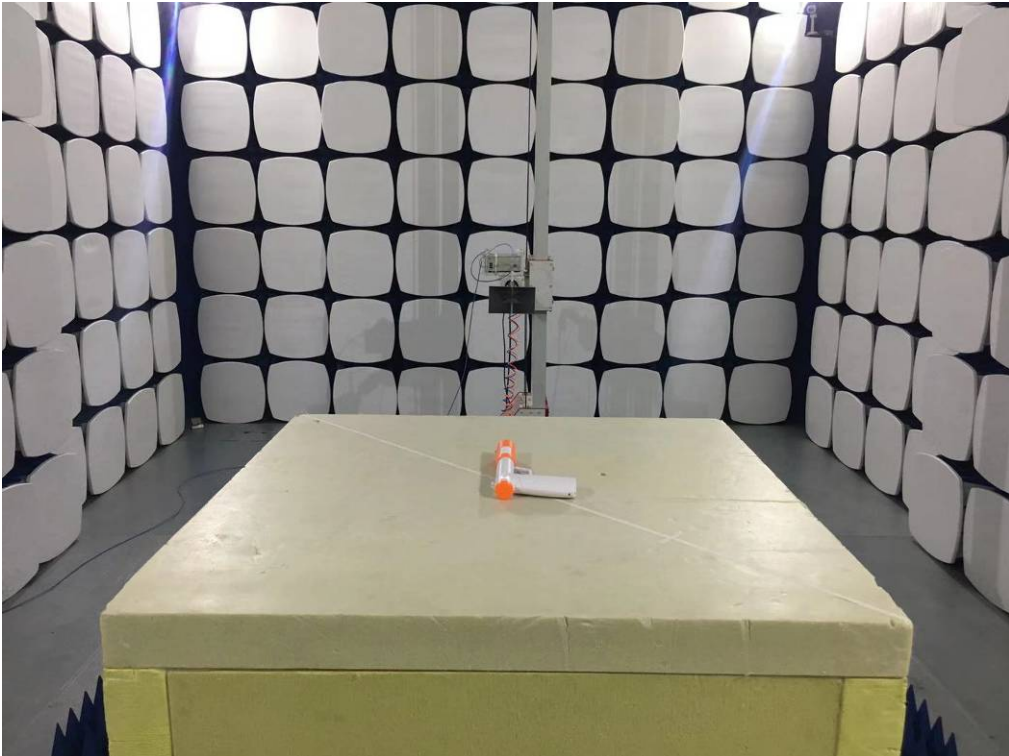
Radiated Setup photo (Above 1G)
