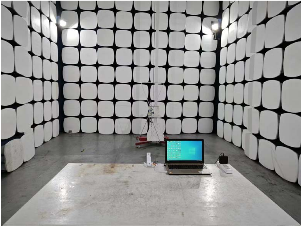
Radiated Setup photo (Below 1G)
