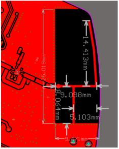
Antenna Module Peak Gain: ~1.5dBi (2 planes tested)
