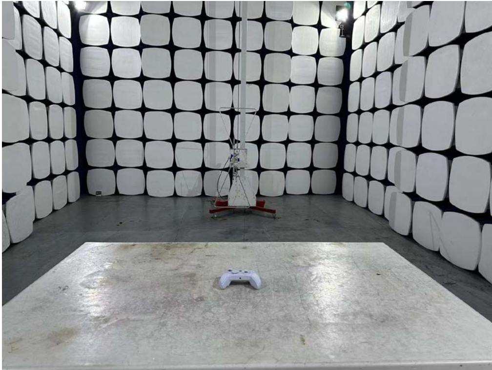
Radiated Setup photo (Below 1G)
