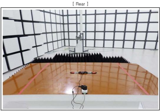
1-3. Setup for conducted disturbance
