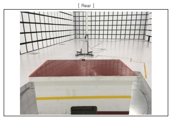
1-2.Setup for Radiated Test: Frequency Above 1 GHz
