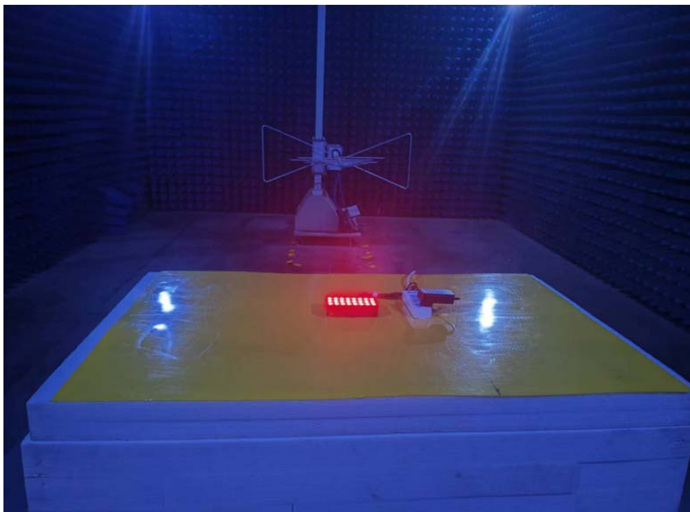
Photo of Radiated Emission Measurement (Above 1G)
