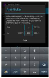
Press the highlighted frequency to enter a custom value between 200 and 1205 Hz.
