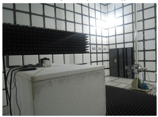
Radiated Emission Set up Photos (Front View)
