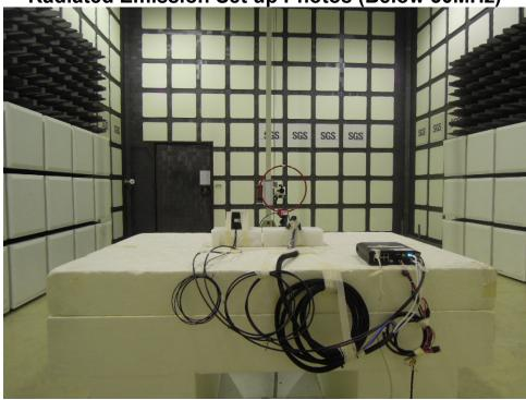
Radiated Emission Set up Photos (Below 1GHz)
