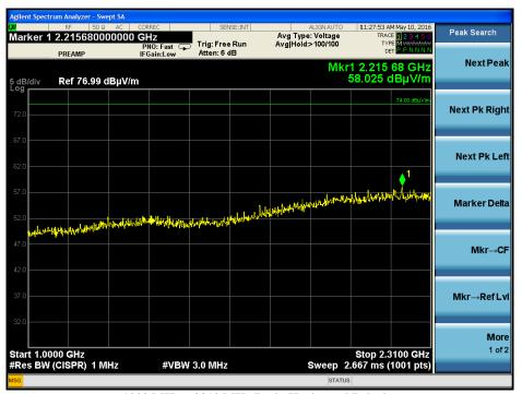
1000 MHz - 2310 MHz Peak, Horizontal Polarity
