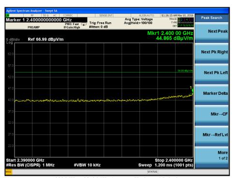
1000 MHz – 2310 MHz Average, Horizontal Polarity
