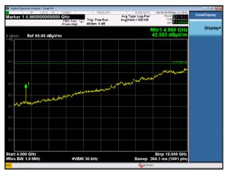
4 GHz – 18 GHz Reduced VBW, High Channel
