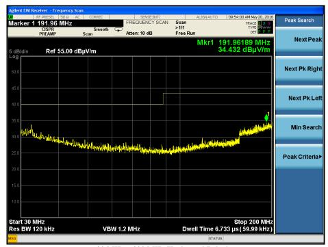
30 MHz - 200 MHz Horizontal Polarity
