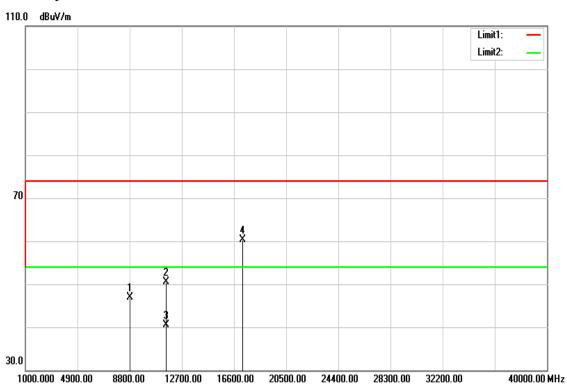
Operation Mode: TX / IEEE 802.11n HT 40 MHz mode / CH Low Test Date: August 25, 2016
