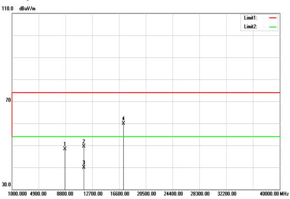
Operation Mode: TX / IEEE 802.11n HT 20 MHz mode / CH Low Test Date: August 25, 2016
