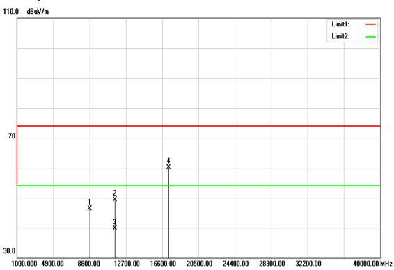
Operation Mode: Tx / IEEE 802.11ac VHT 80 MHz mode / CH Mid Test Date: August 25, 2016
