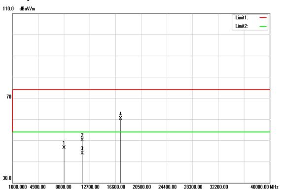
Operation Mode: TX / IEEE 802.11n HT 40 MHz mode / CH High Test Date: August 25, 2016
