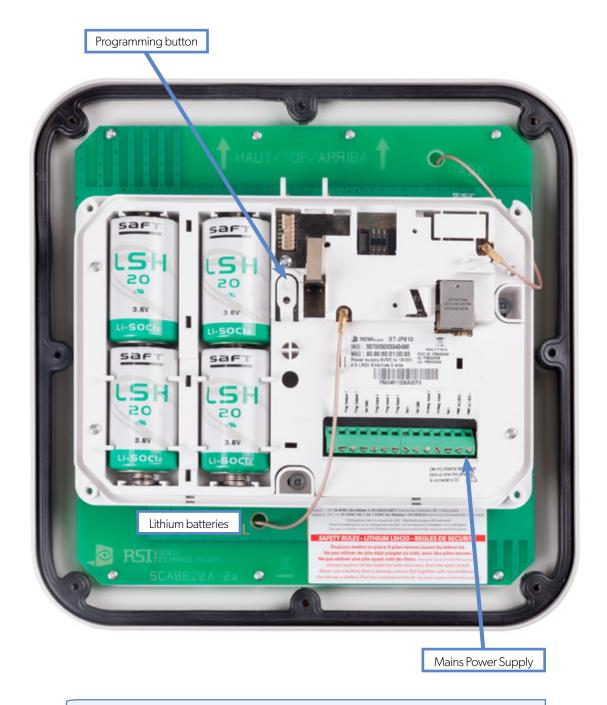
Do not use Lithium batteries when the panel is mains powered When using Ethernet, only power yor panel with the mains power supply.
