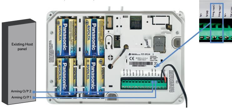
When the panel is used in XTENDER mode, the system will only be able to arm and disarm by latching 9-12Vcc to its arming inputs Arming Input 1 and/or Arming Input 2.
