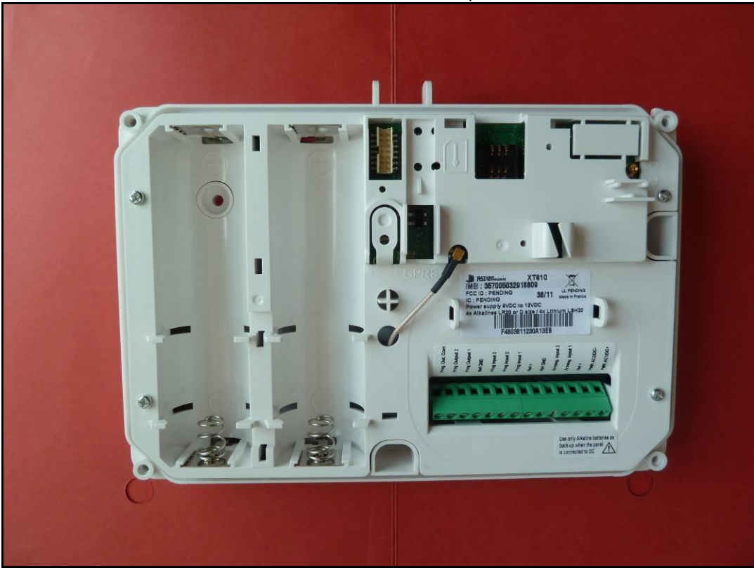
Photo 6: EUT A enclosure opened
