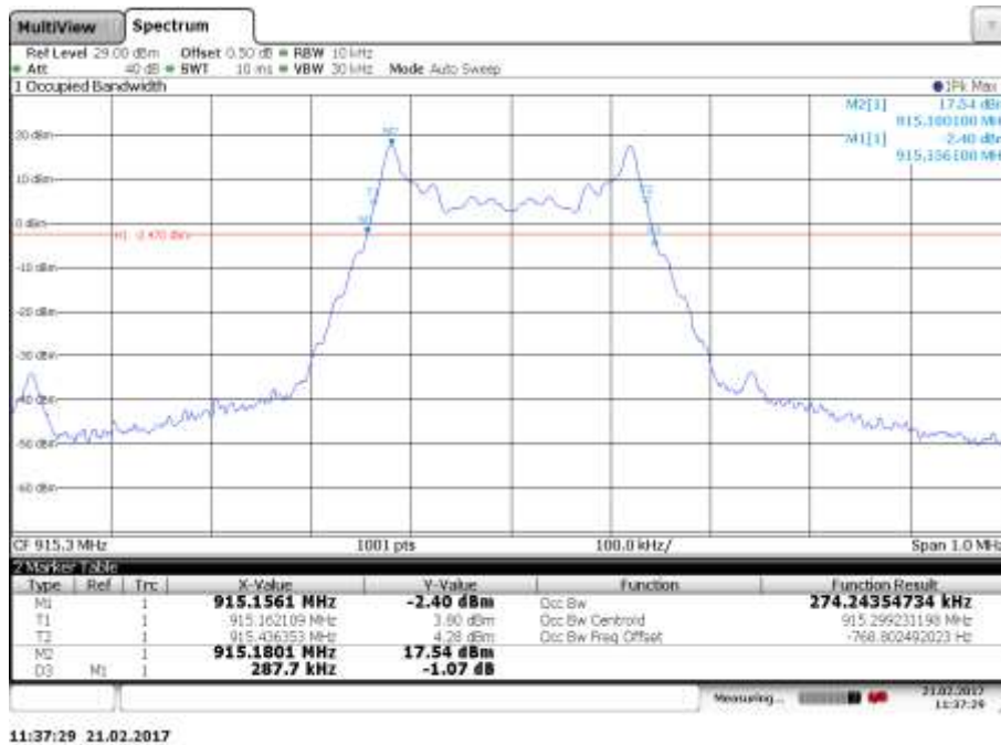
Plot 2: Mid channel; 20 dB bandwidth and 99 % occupied bandwidth
