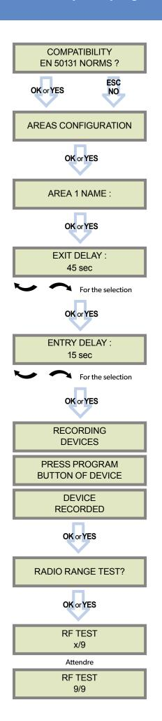
For full compatibility with EN50131 norms, press **OK** or **YES**. Otherwise, press **ESC NO**.
