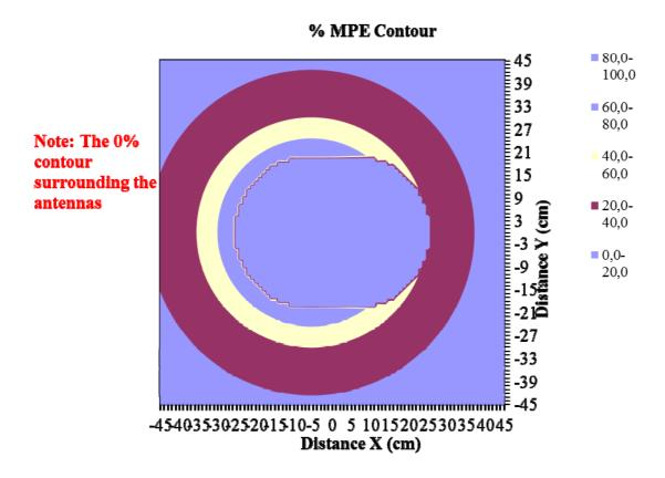
Result: The sum percentage for location that are at least 20 cm from any active antenna is 89.5% and below the Limits for Maximum Permissible Exposure.
