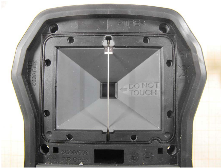
Photo 5: Antenna (normally behind the movement sensor lens)
