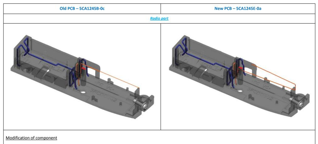
• Size of radio antenna was modified, the new is taller.
