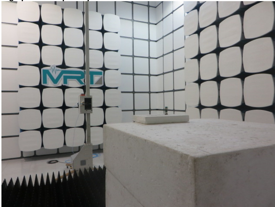
Photograph 3: Set-up for Spurious Emissions above 1GHz
