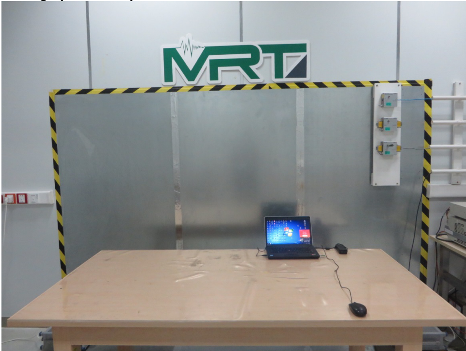
Photograph 4: Set-up for Conducted Emission Test
