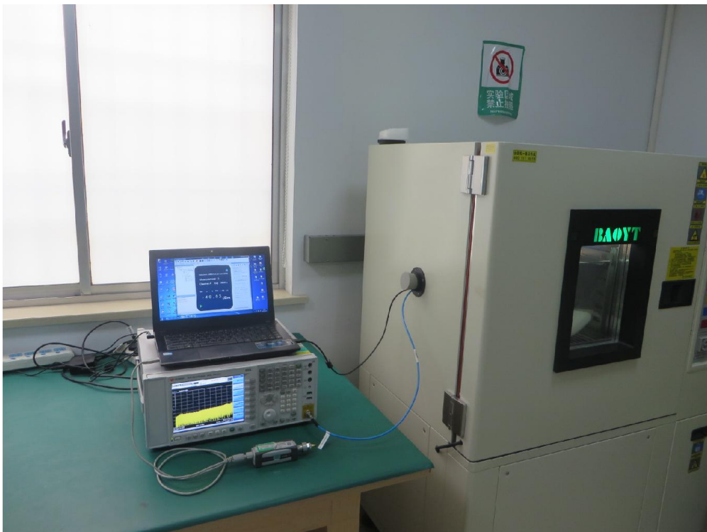
Description: Conducted Emission Test Setup
