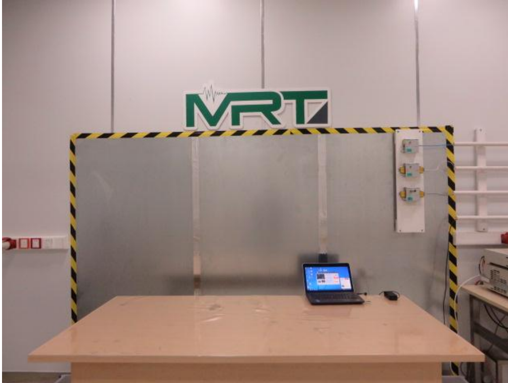
Photograph 1: Set-up for Conducted Emissions
