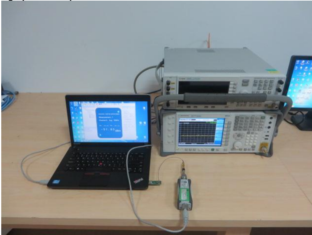
Photograph 2: Set-up for Conducted RF test at Antenna Port
