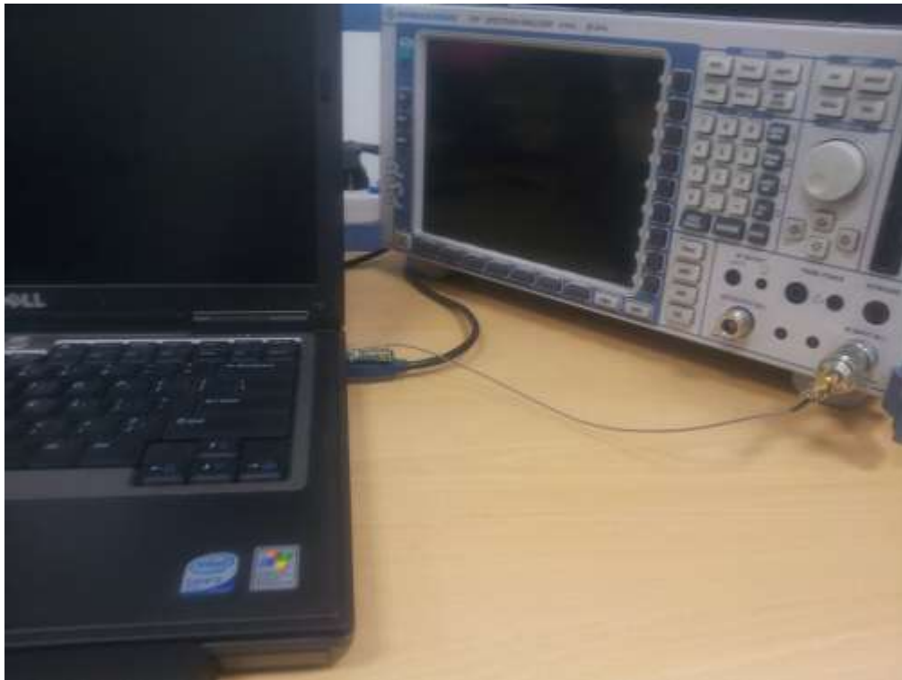
Photograph 1: Set-up for Conducted Power at Antenna Port
