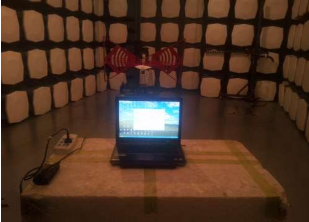
Photograph 3: Set-up for Radiated Emission, 1G-18GHz
