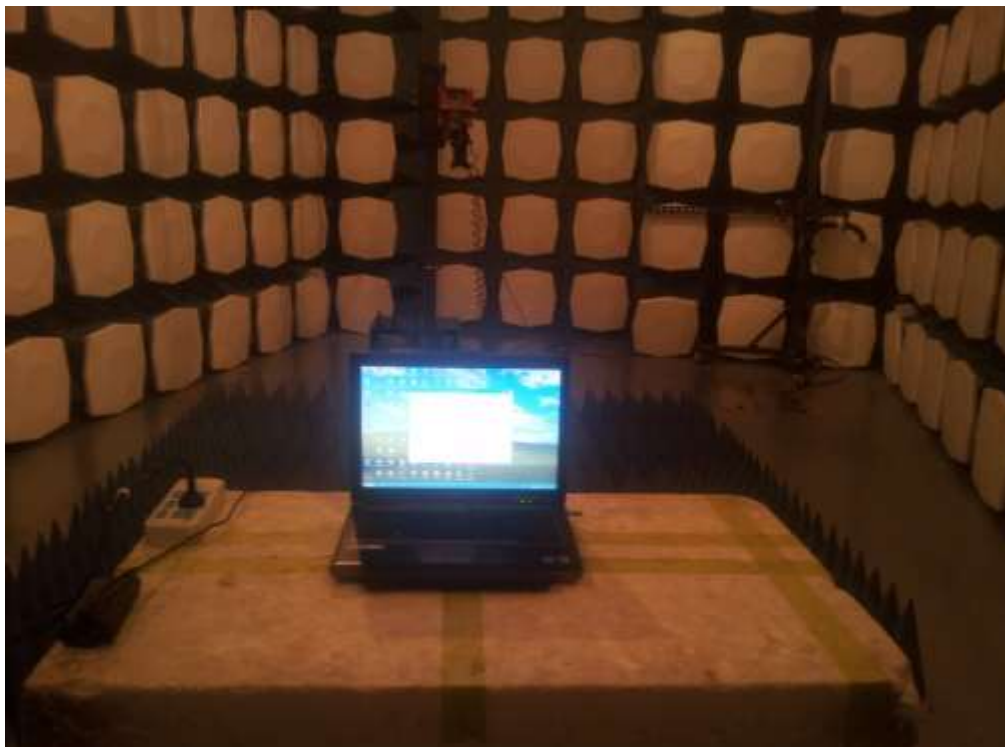
Photograph 3: Set-up for Radiated Emission, 1G-18GHz
