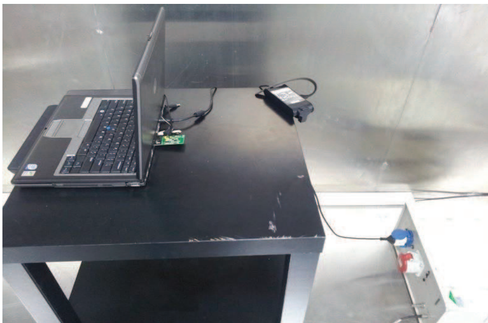
Photograph 1: Set-up for Conducted Emission at Antenna Port
