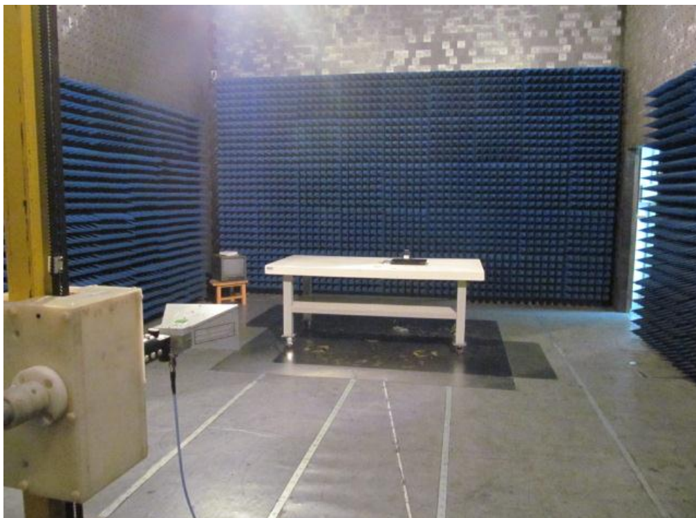
Photograph 3: Set-up for Radiated Emission, 1G-18GHz
