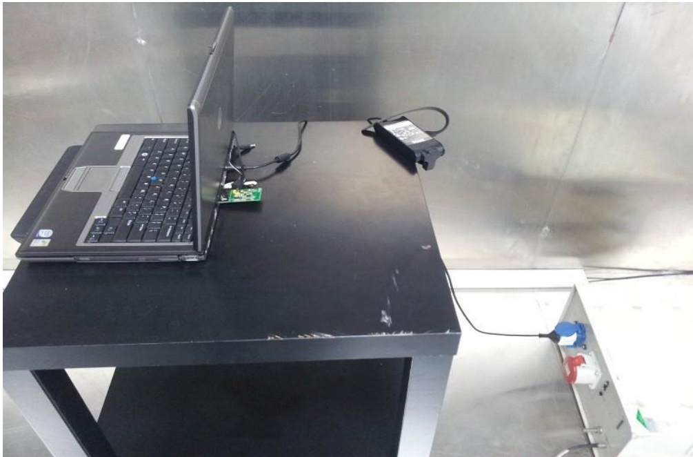
Photograph 1: Set-up for Conducted Emission at Antenna Port
