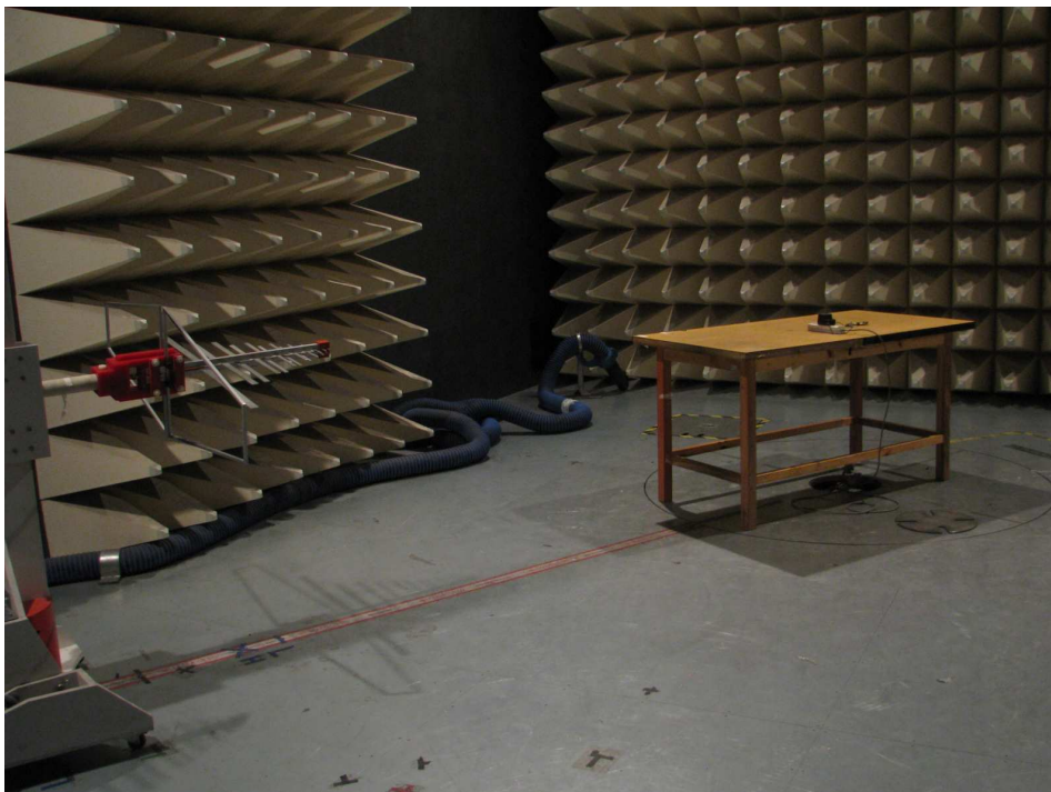
Photograph 3: Set-up for Radiated Emission, 30MHz-1000MHz
