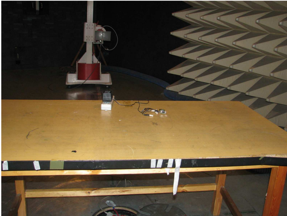
Photograph 4: Set-up for Radiated Emission, 1G-18GHz
