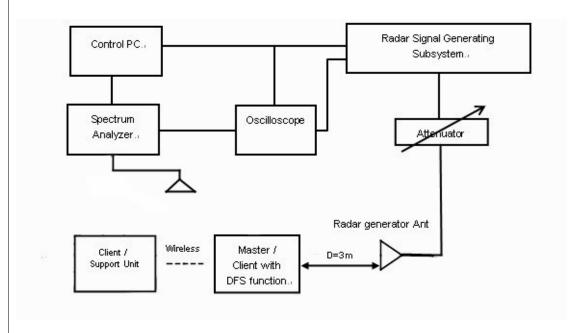
The test transmission will always be from the Master Device to the Client Device. While the Client device is set up to associate with the Master device and play the MPEG file (6  $\frac{1}{2}$  Magic Hours) from Master device, the designated MPEG test file and instructions are located at: http://ntiacsd.ntia.doc.gov/dfs/.
