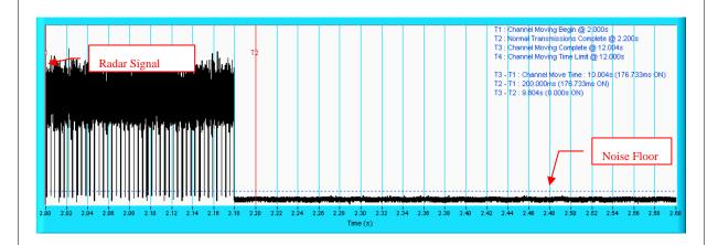
**NOTE:** A Zoom plot for the device vacates the channel in the required 600ms.
