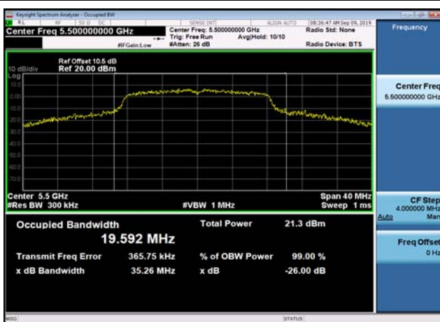
U-NII-2c 99% Bandwidth-802.11a(20MHz) ,5500MHz
