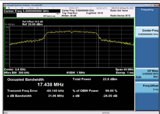
U-NII-2c 99% Bandwidth-802.11a(20MHz) ,5600MHz
