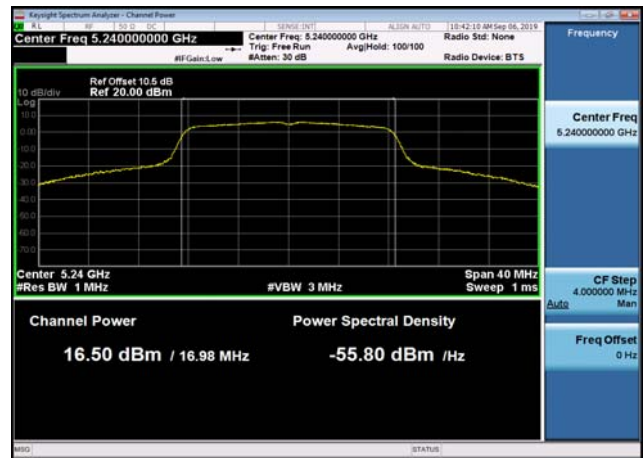
U-NII-1 Output Power-802.11a(20MHz) ,5240MHz
