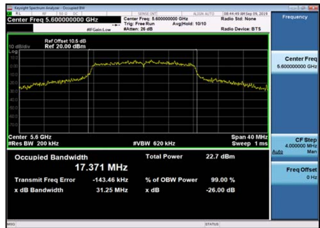
U-NII-2c 26dB Bandwidth-802.11a(20MHz) ,5600MHz
