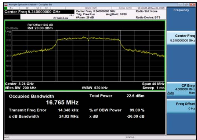
U-NII-1 26dB Bandwidth-802.11a(20MHz) ,5240MHz
