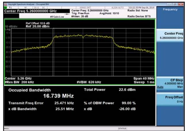
U-NII-2a 26dB Bandwidth-802.11a(20MHz )5320MHz
