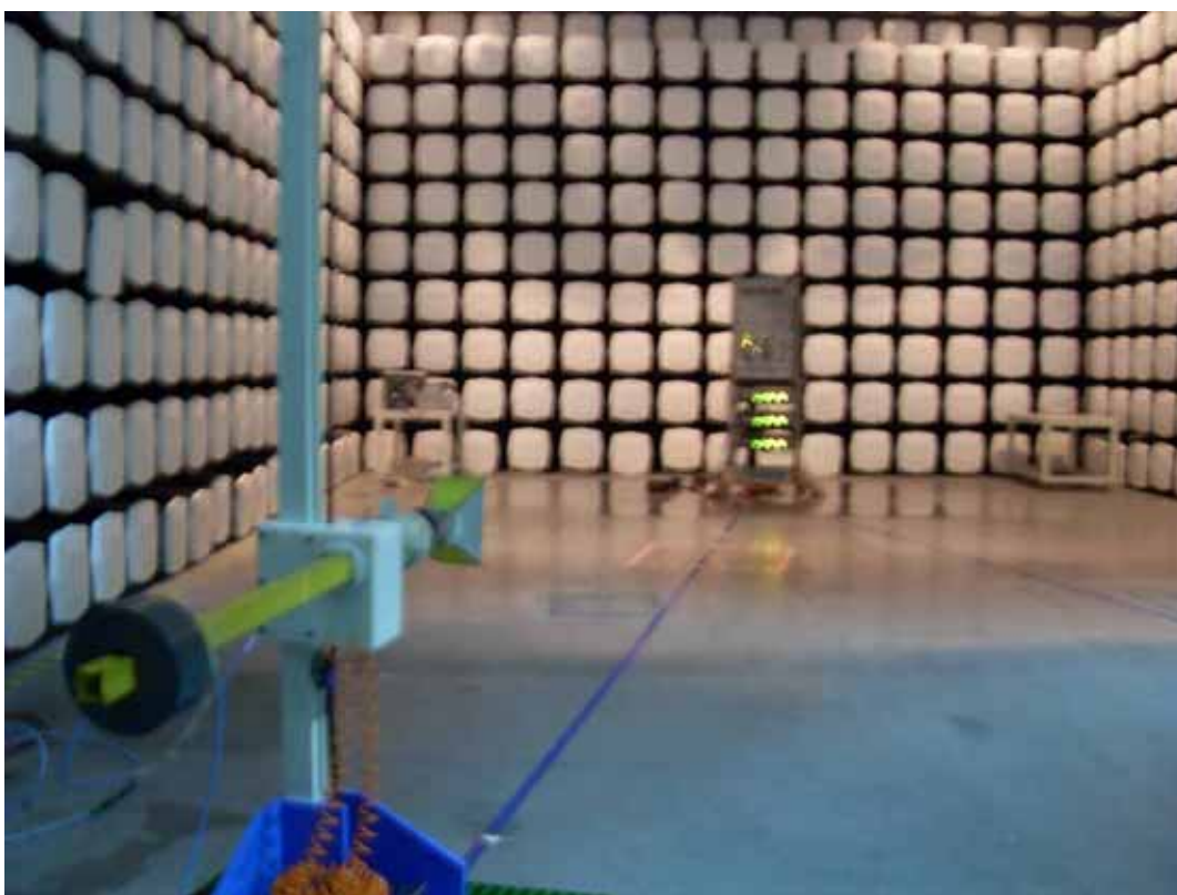
Radiated Emission Test Set-Up 1-10GHz
