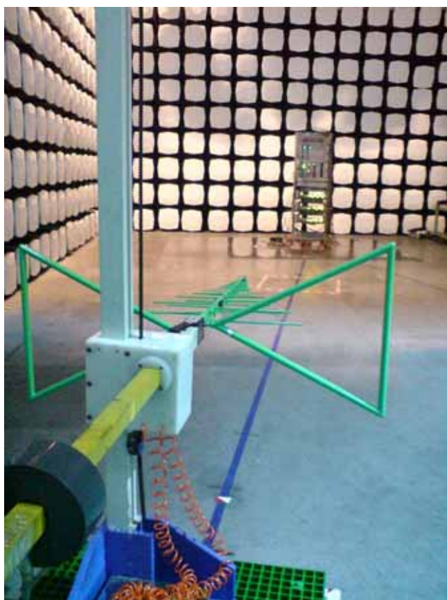
Radiated Emission Test Set-Up 30-1000MHz
