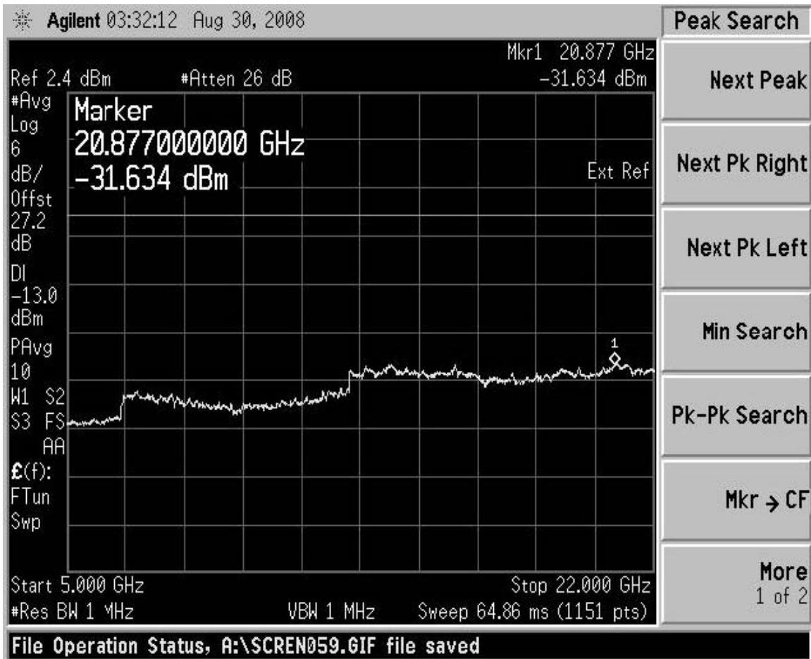
Figure 20: Spurious Emissions - 2 Carriers - Channel 1250, 1275, 5 GHz to 22 GHz
