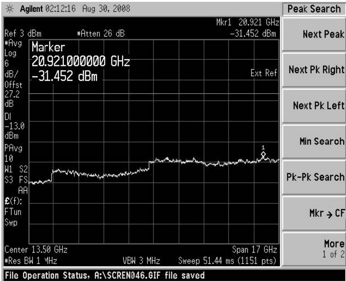
Figure 27: Spurious Emissions - 3 Carriers - Channel 1225, 1250, 1275, 5 GHz to 22 GHz
