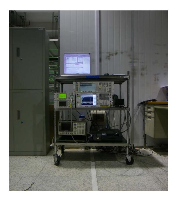
MFRM3 1900MHz Test Setup
