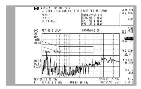
PHASE to Ground Conducted Class B Tabulated Measurements
