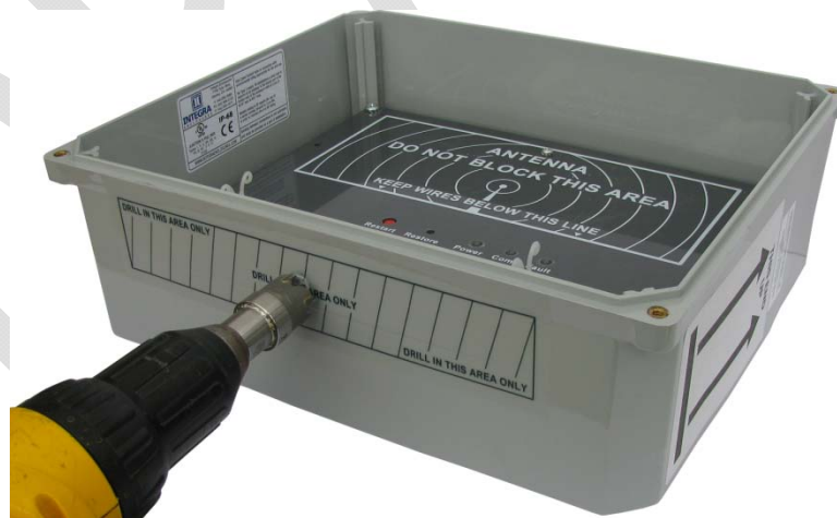
Figure 5: Drill hole for the wire grip within the marked area
