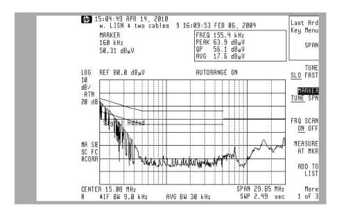
**NEUTRAL to Ground Conducted Class B Tabulated Measurements**
