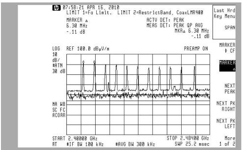
\* Note: Regarding 10 Channel Plot: 11 channels are displayed because the highest channel 255 is not used in slave mode.
