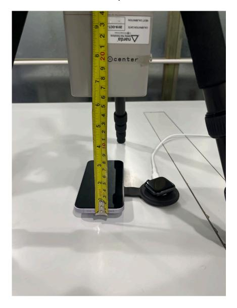
The definition of location for RF exposure test
