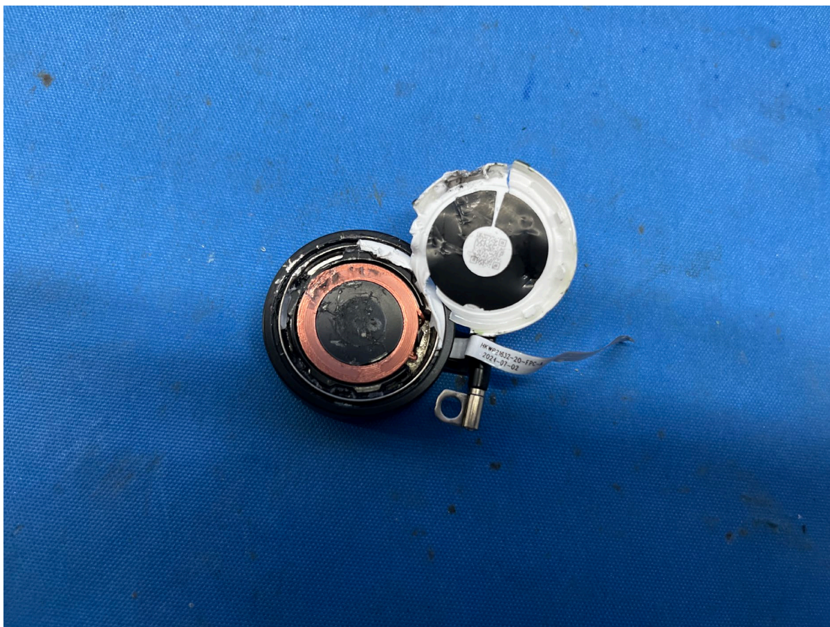
This coil is the smartwatch charge pad
