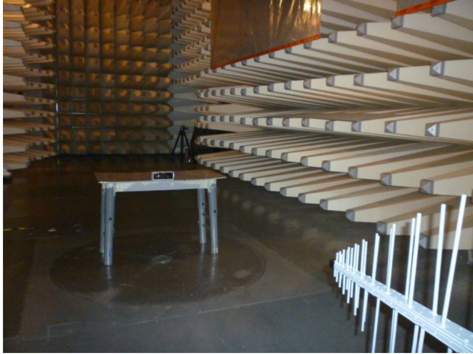
Setup for Radiated Emission
