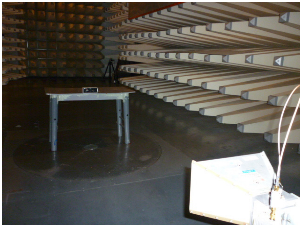
Setup for Radiated Emission
