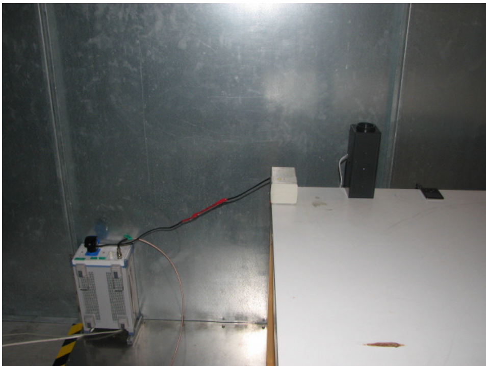
Setup for Conducted Emission
