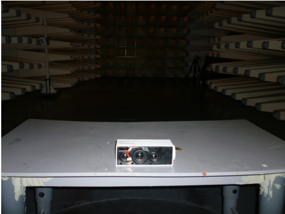
Setup for Radiated Emission
