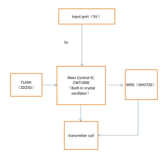
Working principle: The input voltage is 5V, which directly supplies power to the main control IC CWT1000, and then the main control IC starts to work.
