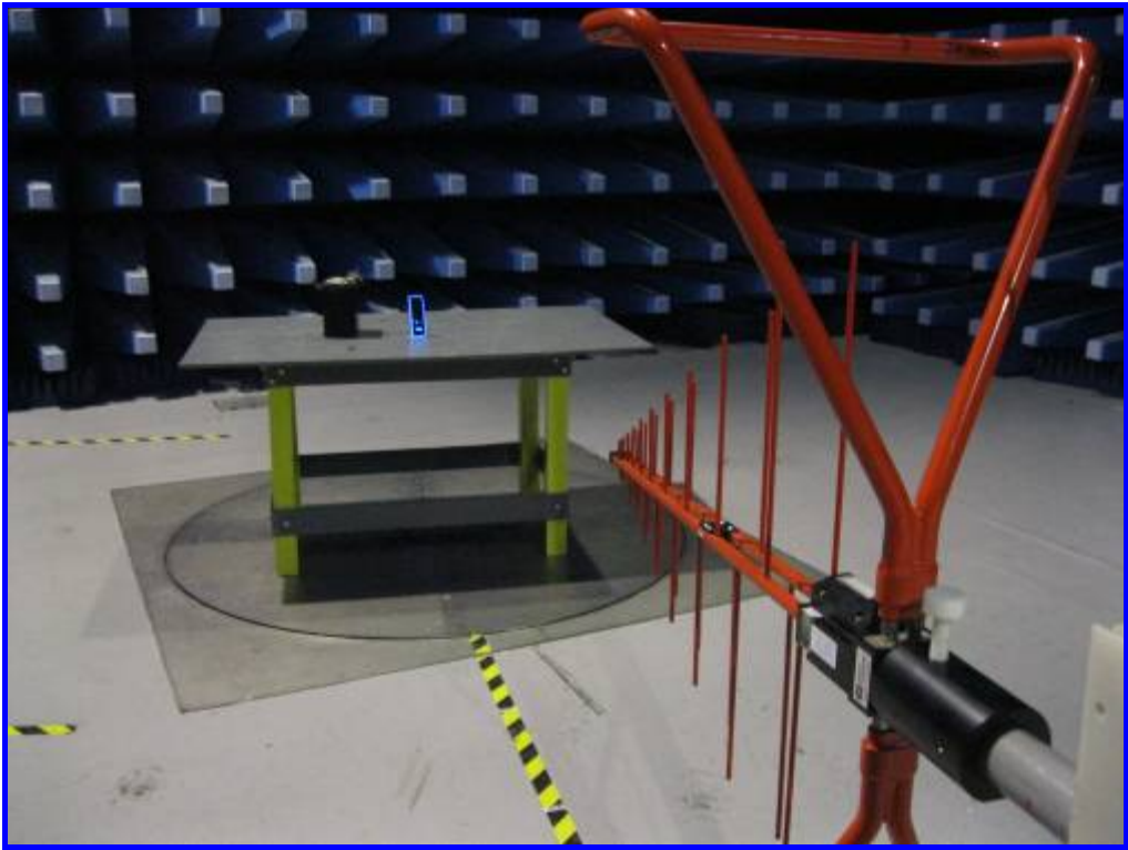
Front View of Radiated Emission Test Setup above 30MHz
